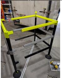
Add the rungs to the ladder half that is secured to the floor
